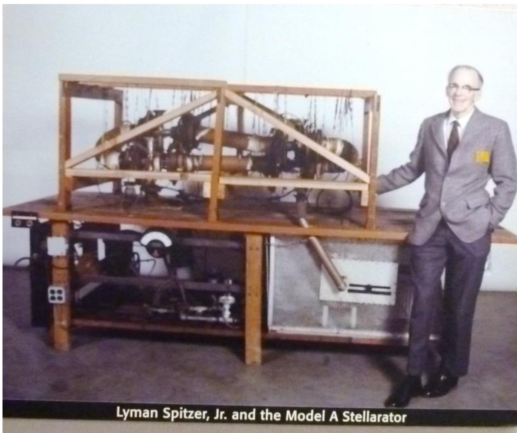
Fig. 2 Lyman Spitzer and his first Stellarator Machine. This was designed only by two theoreticians, Spitzer and Schwarzschild, a son of famous Karl Schwarzschild on Black Hole. They really try to produce the fusion energy with this small machine in 1950's.
